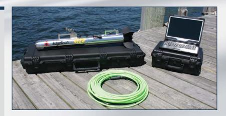
EdgeTech's 4125 Side Scan Sonar System was designed with both the Search & Recovery (SAR) and shallow water survey communities in mind. The 4125 utilizes EdgeTech's Full Spectrum® CHIRP technology, which provides higher resolution imagery at ranges up to 50% greater than non-CHIRP systems. This translates into more accurate results and faster surveys, thus cutting down on costs.
